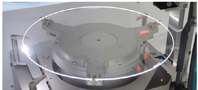
Alignment repeatability 10 \mu m centering/ 0.006° angular; marking speed - 6000 mm/s max; resolution 5 \mu m
